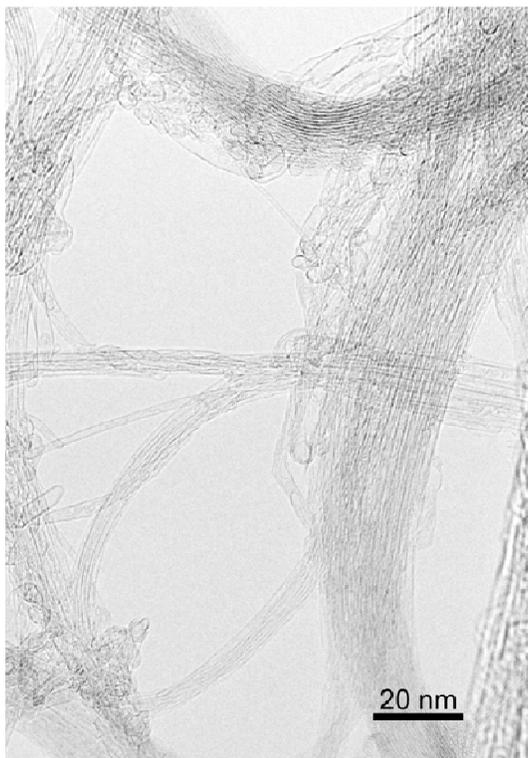
**Figure 1:** TEM image of SWCNTs synthesized from ethanol feedstock. Image captured at an acceleration voltage of 120 kV.
