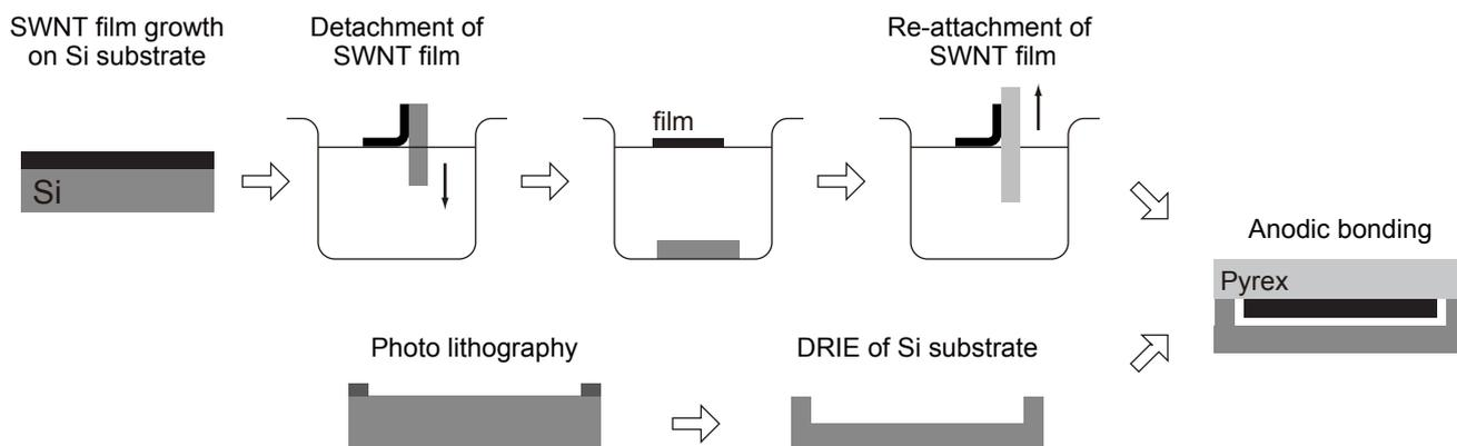
Fig. 1. Fabrication process of the micro gas preconcentrator using an SWNT film. The depth of the Si flow channel was 40  $\mu\text{m}$ , and the volume of the fabricated micro gas preconcentrator was 1  $\mu\text{L}$ .
