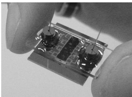
Fig. 2. Photograph of the fabricated micro gas preconcentrator with embedded SWNT film. Deactivated fused silica capillary tubes were connected to the preconcentrator through two holes in the Pyrex glass.
