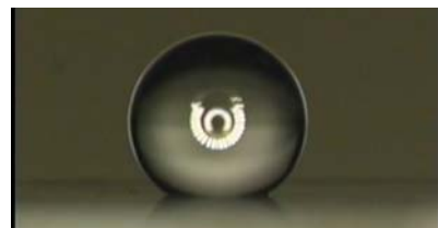
Fig. 2. Picture of water droplet placed on the VA-SWNT film.
