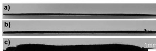
Fig.2 Images of SWNT forests (a) no preheating, (b)preheating: 700 °C, (c)preheating: 850 °C
