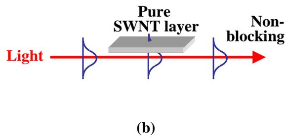
**Fig. 1.** Interaction schemes of the propagating light and nanotubes layers. (a) direct interaction, and (b) evanescent field interaction.
