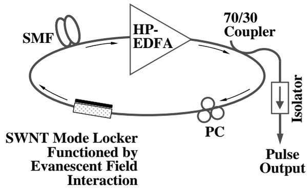
**Fig. 3.** Structure of our mode-locked laser.
