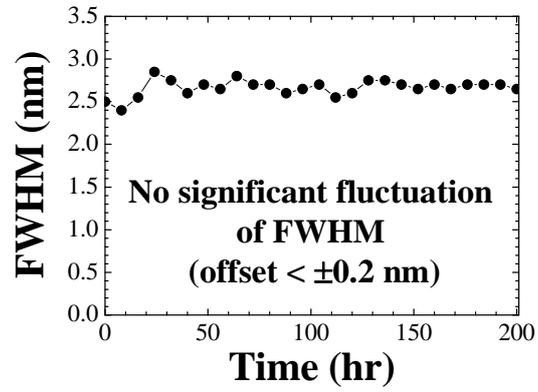
**Fig. 5.** Long-term operation of the pulsed laser. The fluctuation of the FWHM is negligible. Average power is also not degraded showing the negligible fluctuation of  $\pm 0.03$  dBm.
