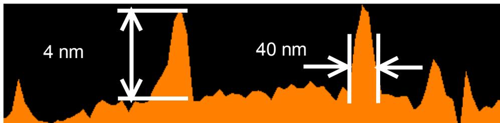
Fig. 3.37 Cross section diagram of SWNT bundles generated on the silicon wafer.
