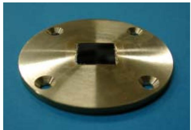
Fig. 3.10 Adapter for heated surface.
