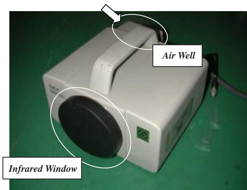
Fig.2.5: Infrared Detector.
