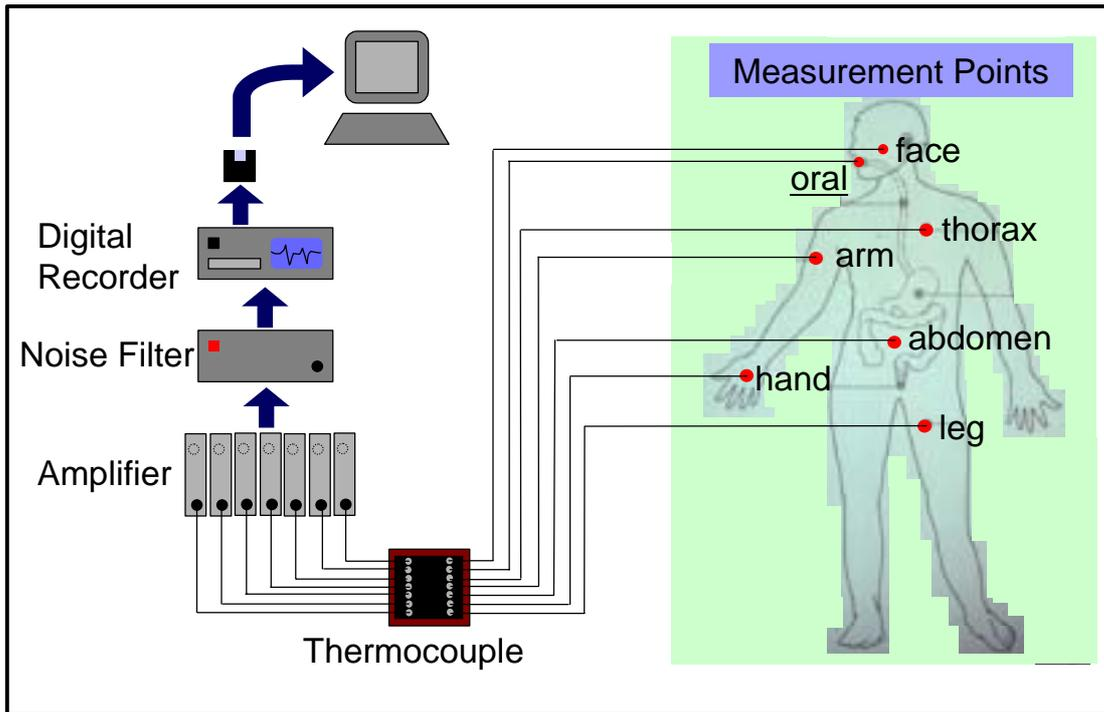
Figure 4.1 Experiment apparatus
