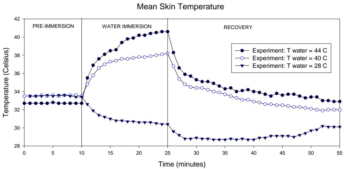
**Figure 5.3 Experiment Results: Mean Skin Temperature of Different Water Temperature Conditions**
