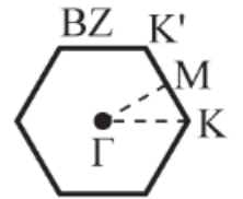
(Top) Graphene structure and geometry. (Left) The Brillouin zone in graphene. (Bottom) The near-Fermi band-structure. The symmetry of graphene leads to the degenerate Dirac points.
