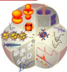
(a) Phonon-phonon coupling throughout the BZ, (b,c) down-conversion pathways, and (d) resulting down-conversion rates. Down-conversion in h-C/BN is nearly identical to that in h-C.
