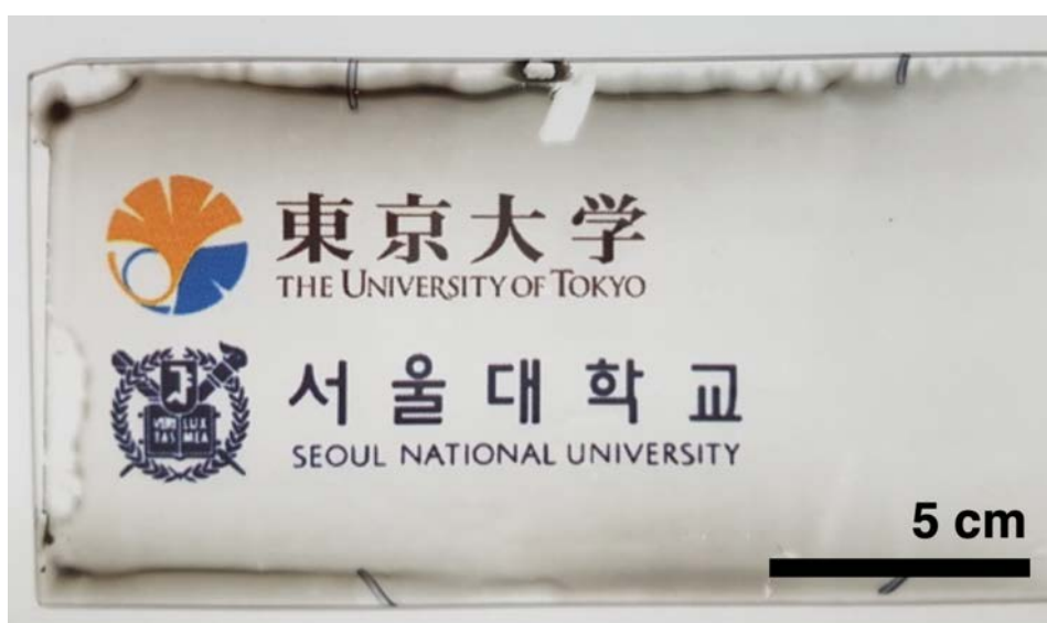
Figure S1. A picture of slot-die coated DWNT electrode on a large glass substrate.
