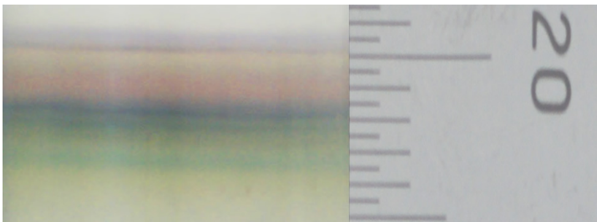
Figure S2. Density gradient fractions with different colors, with mm scale bar (zero is at bottom of the meniscus).
