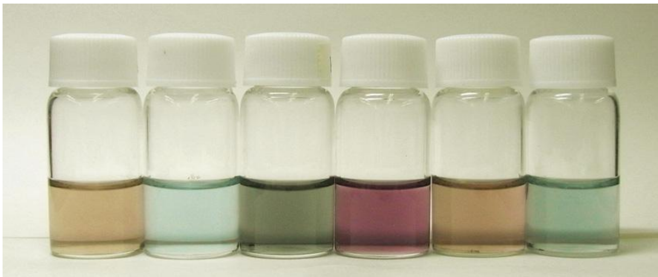
Colors of metallic (M) and semiconducting (S) SWCNTs. From left to right, S and M of LV, S and M of HiPco, S and M of Arc SWCNTs
