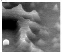
Fig. 4. The type (III) wetting behavior of the VA-SWCNTs during vapor condensation observed
