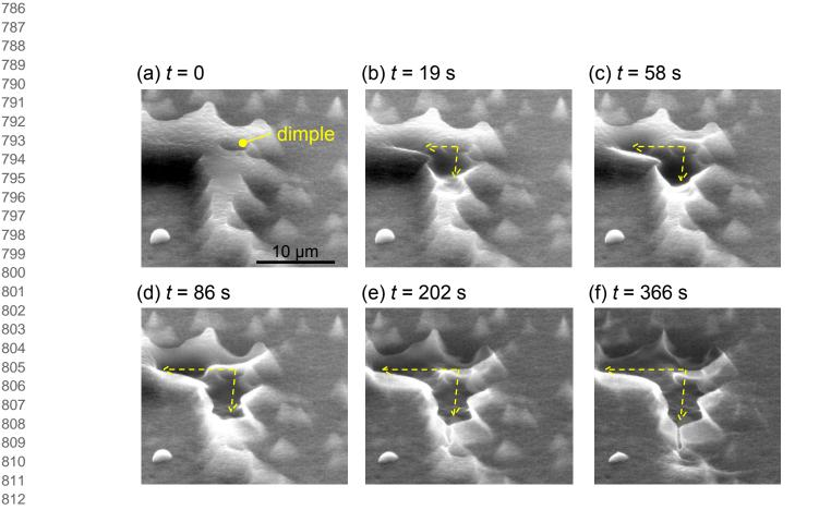
**Fig. 5.** Time evolution of dewetting-induced deformation of the VA-SWCNTs during evaporation of an extensively distributed water layer (the type (III) in Fig. 3) observed in the ESEM chamber having the vapor pressure of  $P \approx 680$  Pa; (a) t = 0 s, (b) t = 19 s, (c) t = 58 s, (d) t = 86 s, (e) t = 202 s, (f) t = 366 s. The dashed arrows in (b)–(f) represent the directions of
