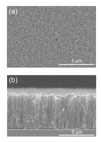
**Fig. 1.** Scanning electron microscope (SEM) images of the VA-SWCNT film from a top view (a) and a side view (b).
