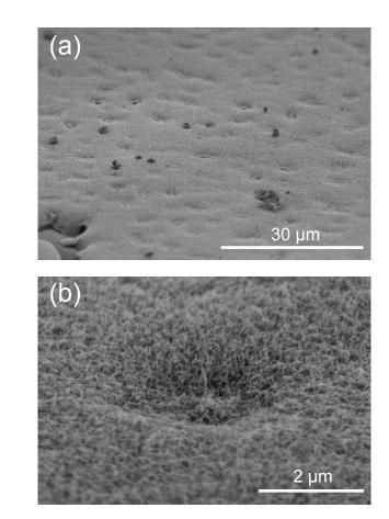
**Fig. 7.** SEM images of the SWCNTs where the water aggregates of types (I) and (II) were present in Fig. 3. The SEM observation angle was 65° in accordance with the ESEM observation (Fig. 2). (a) Dimples distributed on the SWCNT surface. (b) Enlarged view of a representative dimple.
