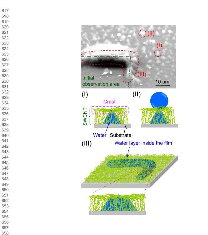
Fig. 3. Wetting behaviors of VA-SWCNTs observed in the ESEM chamber having the vapor pressure of  $P \approx 760$  Pa. Water aggregates under the crust layer were visible because of high porosity of the VA-SWCNT film. Three types of wetting behaviors were exhibited, i.e., (I)
