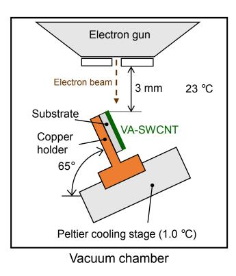
**Fig. 2.** A schematic presentation of the ESEM measurement system. The sample was mounted on a copper holder in contact with a cooling stage at 1.0 °C via a Peltier cooling system. The sample was tilted by 65° with respect to the horizontal direction. The ambient temperature inside the chamber was about 23 °C. Dimensions are not to scale.
